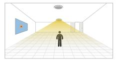
When the person leaves the sensing range, it will automatically turn off the lights after a few minutes.
